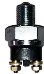
SW361009 NEUTRAL SAFETY SWITCH (CAT) RATED – 24 V BODY – EN1, BASE – PBT GF TERMINAL – BRASS LIFE - 100000 CYCLES
