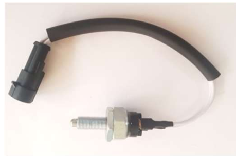
SW3610030 PTO SAFETY SWITCH 12/ 24 V 10 AMP BODY – MS, BASE - PA6 GF 30% LIFE – 50000 CYCLE
